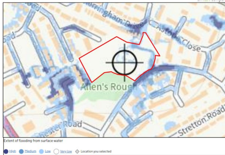
Figure 3 - Map showing the extent of surface water flood risk on the Site, which ranges from very low to medium risk.
