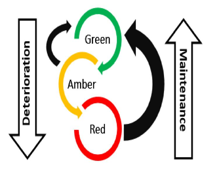
This overview illustrates the principles upon which Walsall's lifecycle planning model is based. Each unit of the asset is classified using a traffic light system, according to its condition. How it is classified is dependent upon the particular asset in question. For carriageways, for example, the asset is classified according to the results of road condition surveys, which are regularly conducted.
