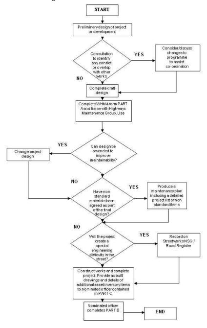
Figure 1 Designing with maintenance in mind and monitoring flowchart
