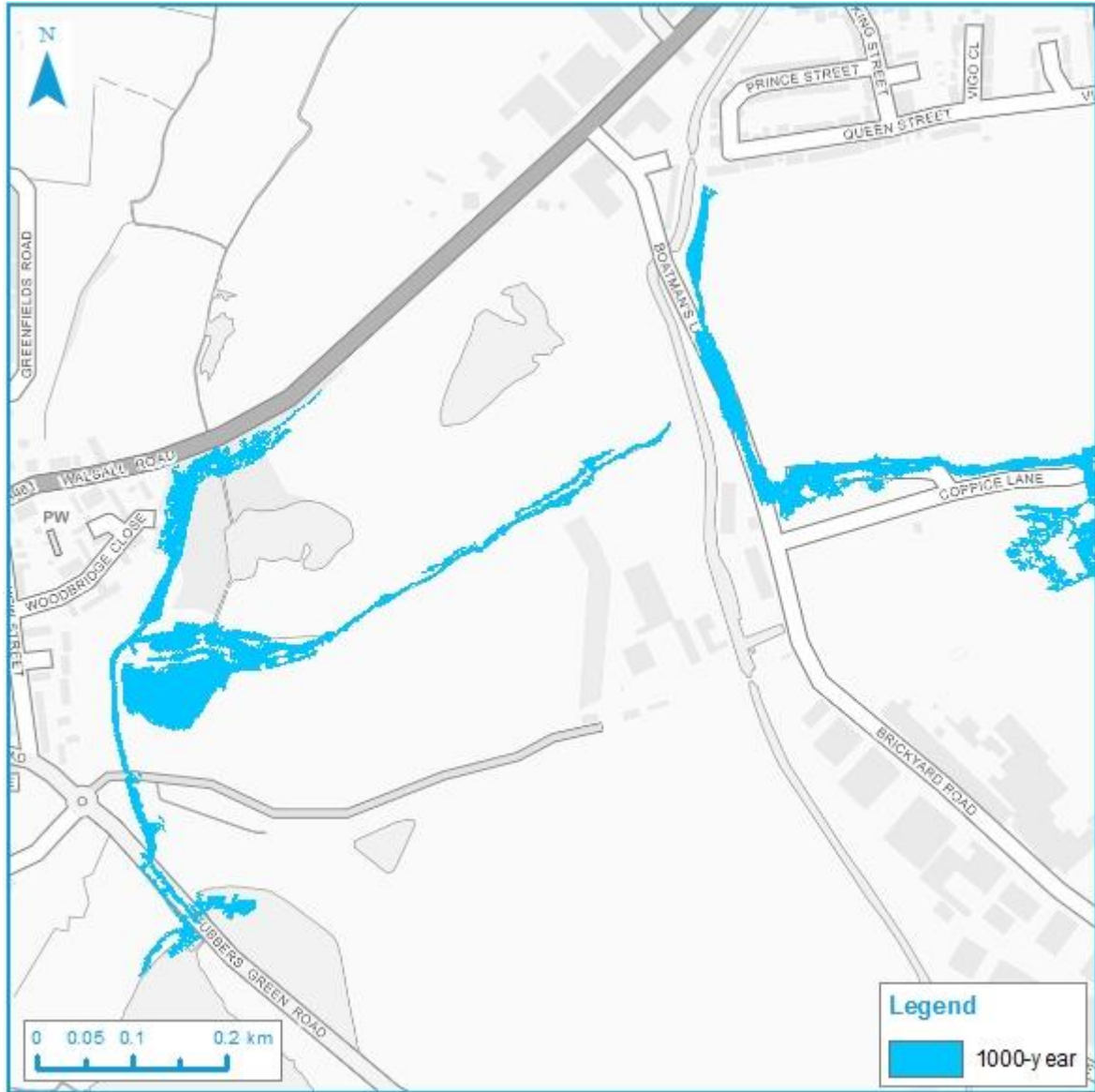
Figure 3: 1000-year flood extents at Highfields South Landfill Site (post restoration ground levels)
