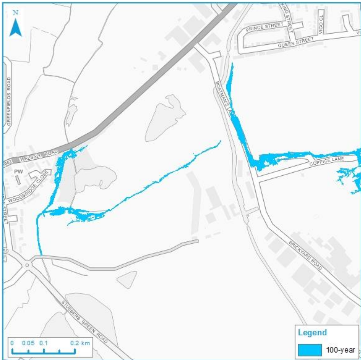
Figure 2: 100-year flood extents at Highfields South Landfill Site (post restoration ground levels)
