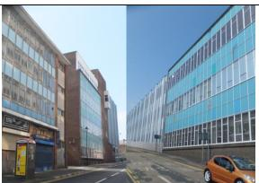
The area is predominantly constructed using reinforced concrete framing. Buildings east of Goodall Street typically frame this in yellow brickwork and infill floors with blue composite spandrel panels and metal frame glazing. The concrete frame and the roof are one structural element and overhanging canopy roofs of painted concrete are typical.
