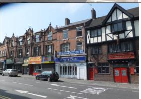
The area comprises a diverse mix of building materials. Red brick is the main facing material and is typically dressed in either stone, blue brick or faience.
