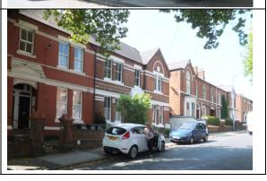
Buildings are all built in the local red clay brick of the town, which has a semi dense fireskin and are dressed in blue brick and sandstone. Roofs are covered in Welsh slate
